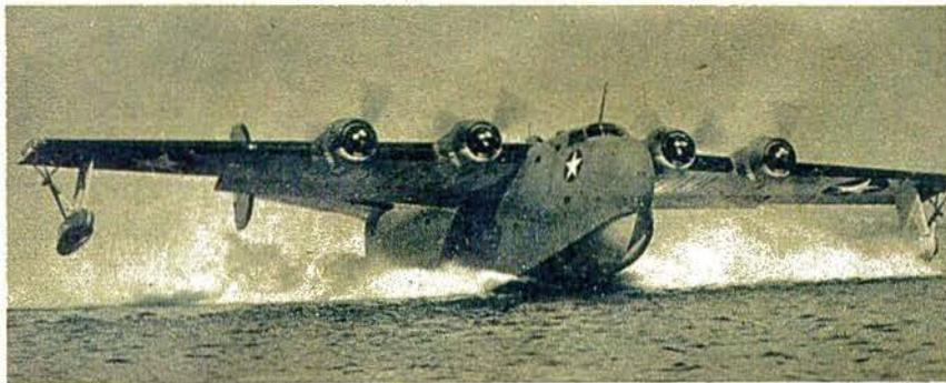
**PB2Y CORONADO**, the giant flying boat of Consolidated Aircraft Co., is equipped with four 4-blade Curtiss Electric hollow steel propellers.
